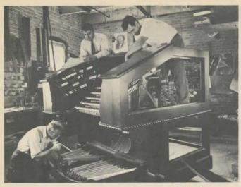
5-manual console nears completion in Moller factory.
