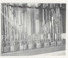
THROUGH THE 'LOOK-IN' GLASS-View through the swell shutters of the Prideaux-Brune organ shows (front to rear) Fagot, Open Diapason, Salicional and Tibia Clausa, with the 16' Tibia pipe in the rear. The white object at the right is a muffler over the tremulant, the entire unit being mounted on top of the sound-dampening blower housing which is within the chamber.
